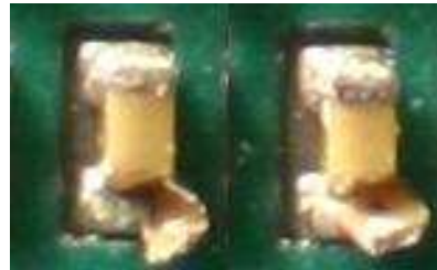
Fig4. Termination exploded due to excessive force applied during placement
