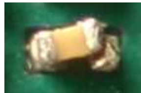
Fig5. Skewed component due to inaccurate placement
