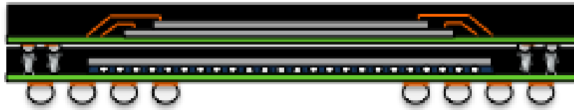
Figure 3. Package-on-Package (PoP) (Example source: IPC-7091)
