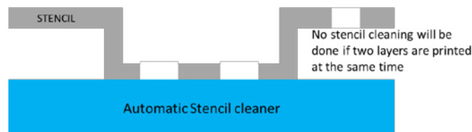
Figure 10 – Automatic Stencil Cleaning Issue with One Pass
