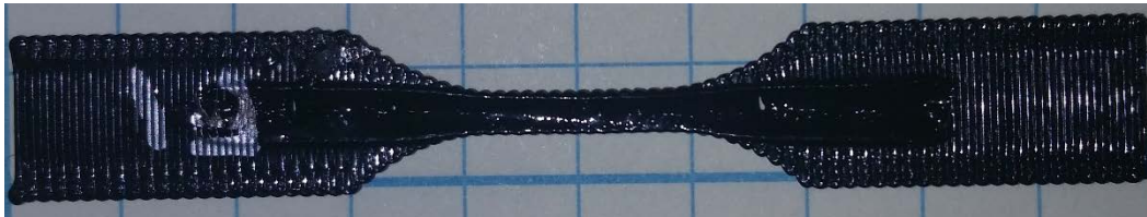
90° Tensile Specimen after Laser Reflow
