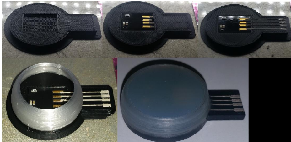
Figure 6: Steps of a Printed USB Device
