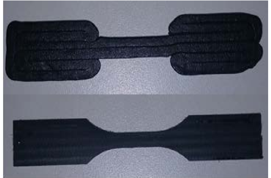
90° Printed and Milled Tensile Specimen
