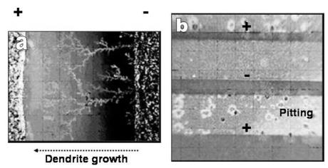
Figure 8. Corrosion problems due to electric filed between conducting lines on a PCB: (a) silver dendrite formation due to migration and (b) pitting between copper conducting lines [13].
