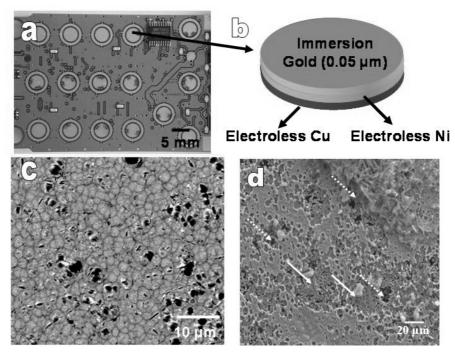
Figure 10. Cell phone key-pad system and galvanic corrosion: (a) key-pad, (b) schematic of the layers on key-pad, (c) microstructure of the gold layer, and (b) corrosion of the key-pad in chloride solutions.
