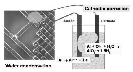
Figure 9. Schematic of the possible cathodic corrosion problem for aluminium conducting lines on ICs.
