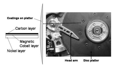
Figure 5. Computer hard disk with description of components [4].
