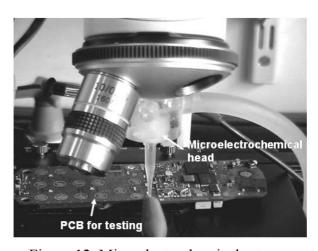
Figure 12. Microelectrochemical set up.
