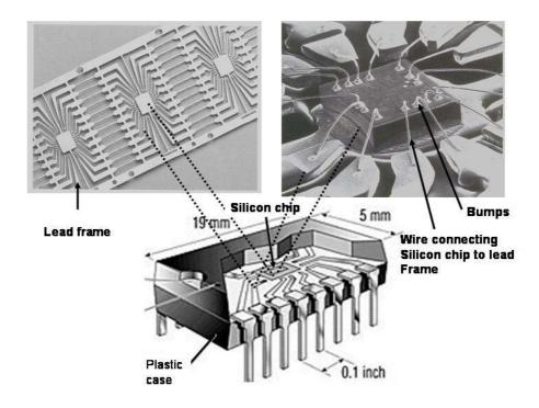
Figure 1. Integrated circuit and related components [2].
