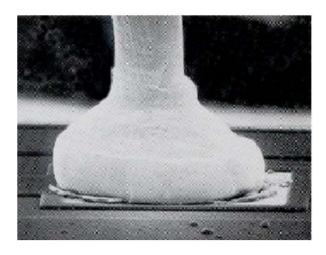
Figure 2. Picture of a ball bonded gold wire to aluminium on an IC circuit
