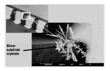
Figure 7. Formation of silver sulphide on a silverpalladium film on exposure to H<sub>2</sub>S [10].
