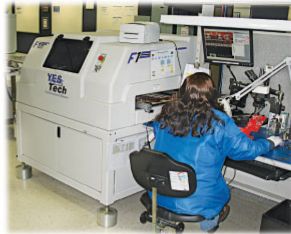
Biamp Surface-Mount Assembly With AOI Inspection
