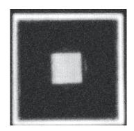
Figure 11. TPA-1 after JEDEC L3 + 3 x  $220^{\circ}$ C IR + 1000 temperature cycles.
