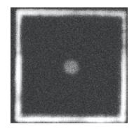
Figure 10. Silicone TIM on Ablestik laminate test package after 1000 temperature cycles.
