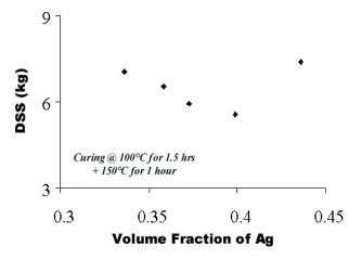
Figure 7. Die shear strength vs. silver loading for TPA-1. *Modulus*
