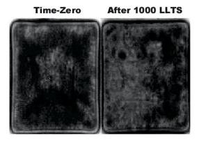
Figure 8. PCM on an 8 x 8 mm die before and after temperature shock. Picture Courtesy of Universal Instruments.
