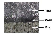
Figure 5. A void at the interface between the TIM and die.
