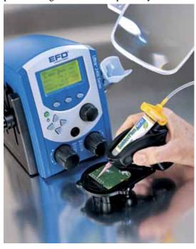
Compared to the use of wire solder and solder preforms, dispensing solder paste with air pressure is a relatively simple and much more flexible option. One would think that with only two machine variables needed to control dispensing, air-powered application of solder paste would be foolproof, but this is not the case.
