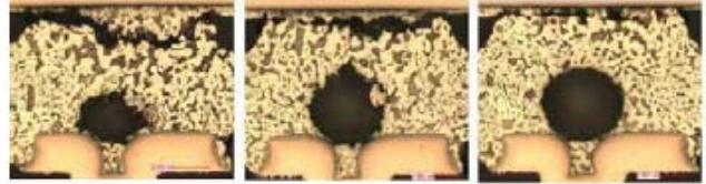
ENIG 2x Reflow – Examples of solder fatigue cracking without void interaction
