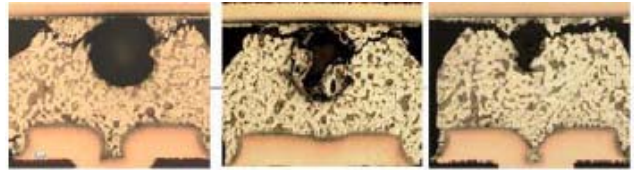
ENIG 1x Reflow – Examples of void-assisted solder fatigue cracking
