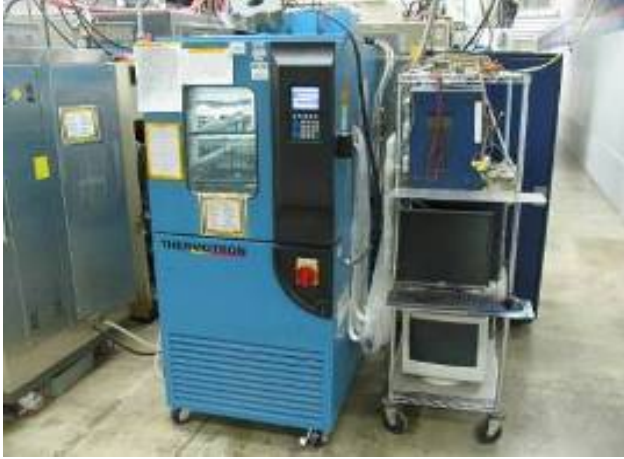
Figure 12. Thermal Cycling Chamber and Anatech
