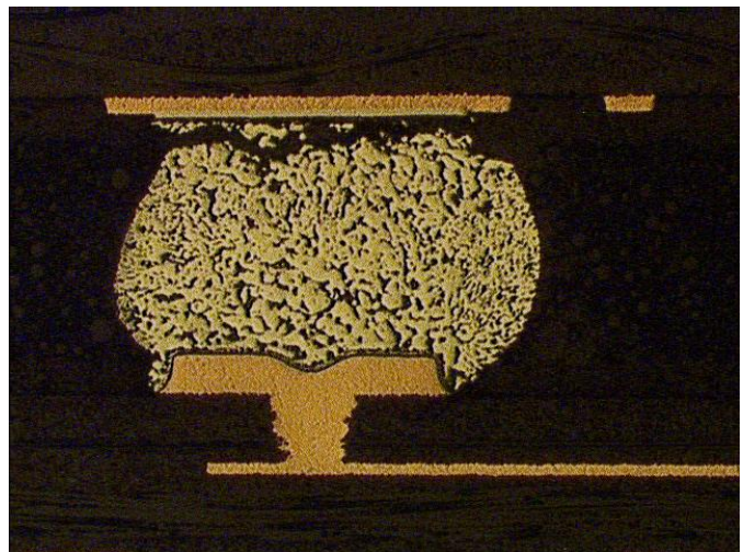
Figure 23. Macro (Top) and Magnified (Bottom) Views BGA Void Assessment: No Void, Outer Row, 311 Cycles, BGA256
