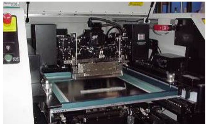
Figure 9. MPM Stencil Printer
