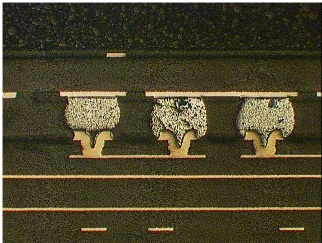
Figure 29. Macro View, BGA56 U1 Component Cross-section Showing Assembly Induced Solder Joint Defect, Failed @ 18 Cycles, BGA 56
