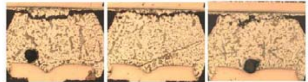
IAg 1x Reflow – Examples of smaller voids and solder fatigue cracking without void interaction
