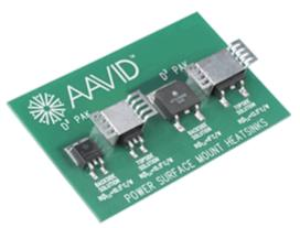
Figure 4. Power devices are fitted with low-profile surface mounted heat sinks.
