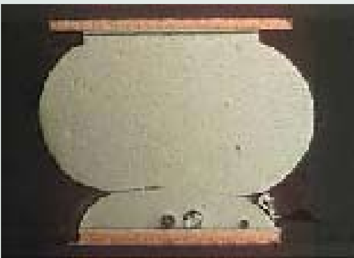
Figure 7 - An example of “head-in-pillow” defect.
