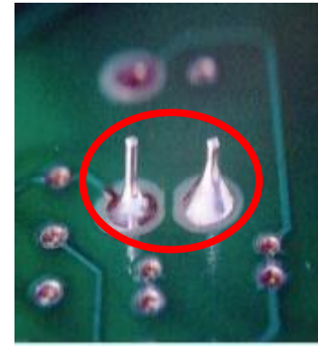
High welding spot without coating
