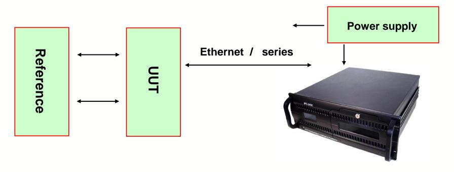
BIST for DSL test only requires power supply and IPC (industrial PC), reference unit provides BIST software support, so it needn't redesign UUT (unit under test) adding extra logic chips and memories; UUT performs shelf-test by getting controlled from IPC and download synchronous software from the reference unit.
