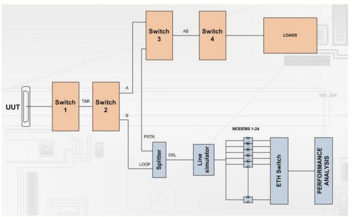
External test instruments are connected together through wire, and controlled by controller through GPIB, series or ETH, which is more easier to generate false reject.
