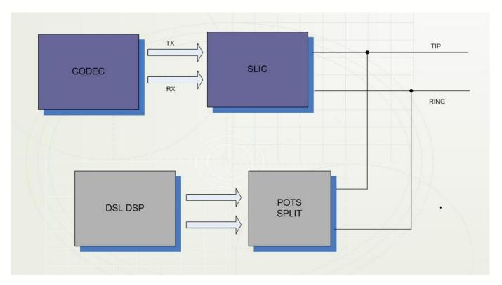
The figure above is a representation of the basic functional components. This refers to the DSL section (DSP and POTS) tests require that tip and ring be unterminated. The tip ring supply is a current source.
