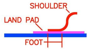
The gull wing lead has a limit as to how much solder volume will wet to the surface. Any excess flows off of the PCB land pad and bridges to adjacent pads, when looking at fine pitch components. The solution is to reduce the volume of solder paste deposited at print.
