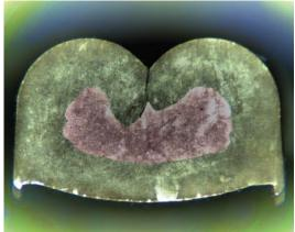
Micrograph analysis of crimped wire
