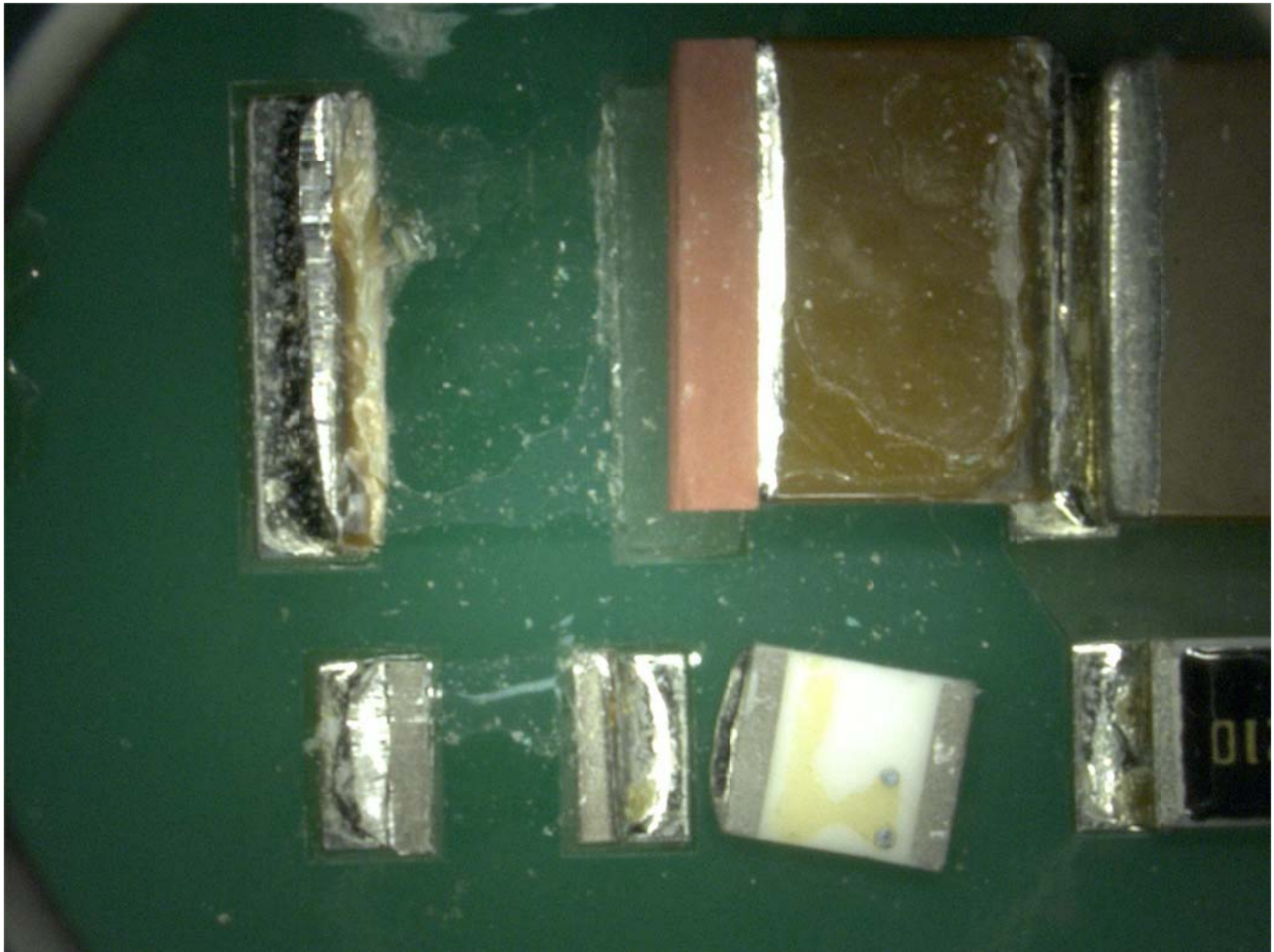
Figure 9: Flux Residues Under the Body of the Component
