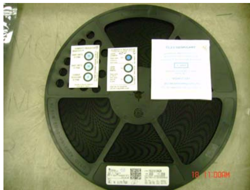
Figure 14 TSC2101IRGZR devices in original tape and reel with 1 desiccant and moisture indicator labels.
