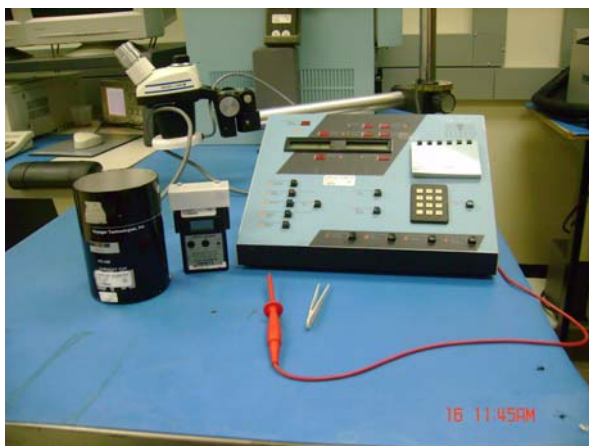
Figure 15 ESD Analyzer with Faraday cup and voltage field meter.
