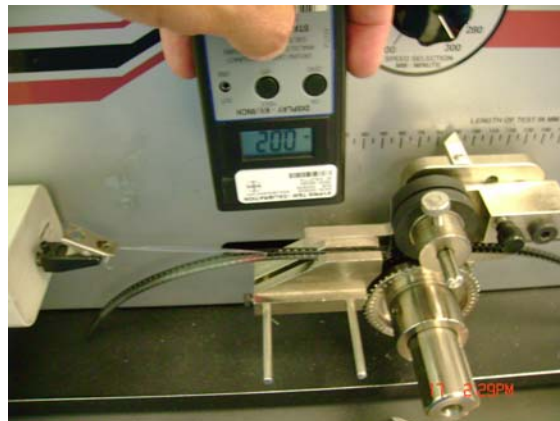
Figure 18 Less than 20 volts detected during measurement of the static charge generated during peel back testing.
