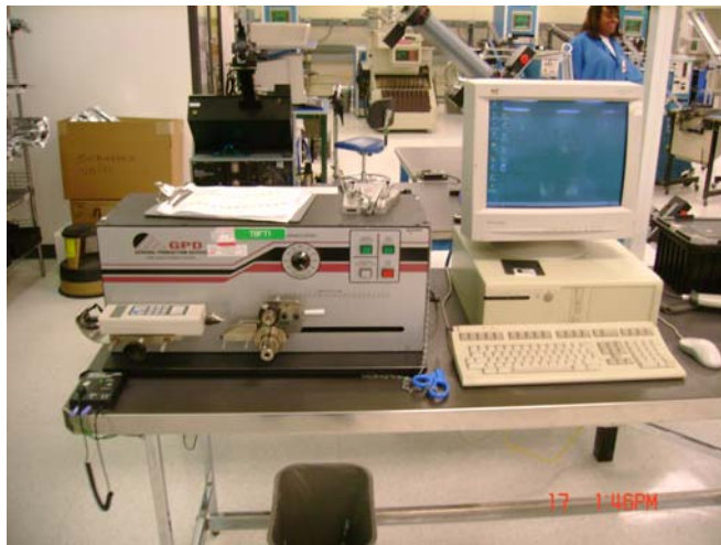
Figure 16 Peel-Back Force Test (PBFT) System.
