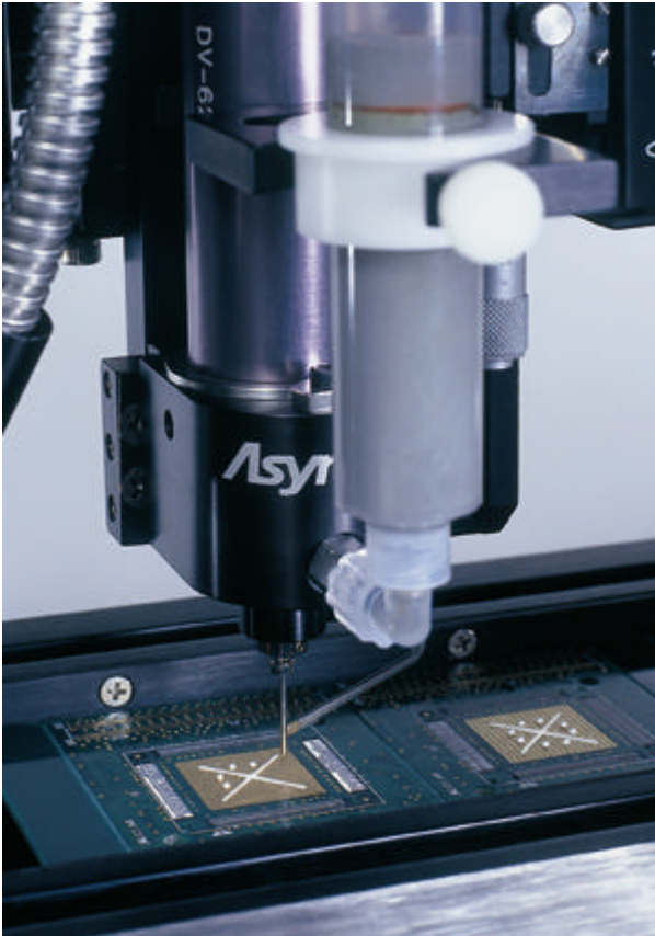
Figure 10. example of large die attach application.
