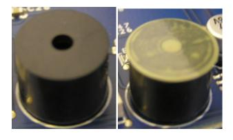
Figure 1: Is the component sealed at the base as well as at the top for conformal coating leaking?
