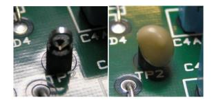
Figure 4: Masking of a test point with Liquid Latex is simple and seals very effectively
