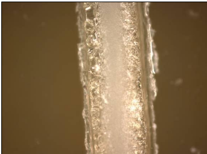
Figure 4. Close up of flux residue on conformal coating
