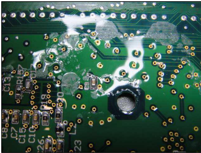
Figure 1. Blisters immediately appeared with this combination of flux and coating.
