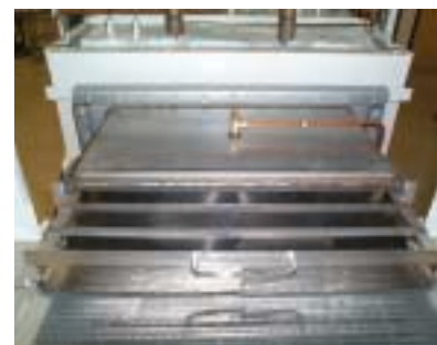
Fig 4 Gas curtain used to keep outside air from the furnace
