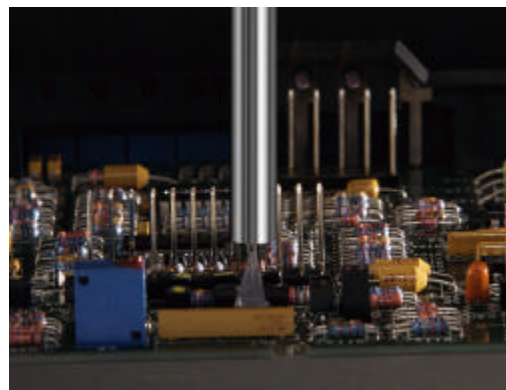
SwirlCoat applicator dispensing in "swirl-spray" mode
