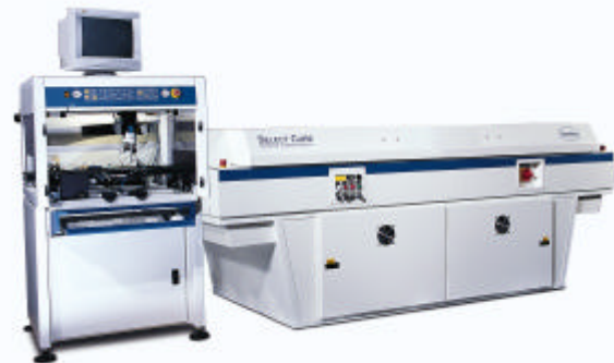
In-line Infra-Red Coating/Curing System
