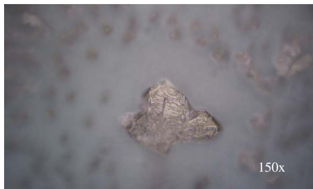
Figure 5 – Inside ESD bag surface above capacitor #2
