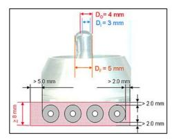
Figure 4 – Minimum required clearance for single miniwave processes
