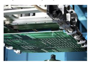
Figure 1 – Single nozzle miniwave process
