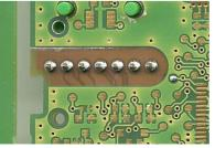
Figure 11 - Avoid solder resist close to the solder joint
