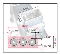
Figure 3 – Minimum required clearance for multi-nozzle dip processes
