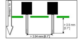
Figures 8 – Multi-nozzle dip soldering: pitch and lead length
