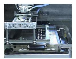
Figure 2 – Multi-mozzle dip process
