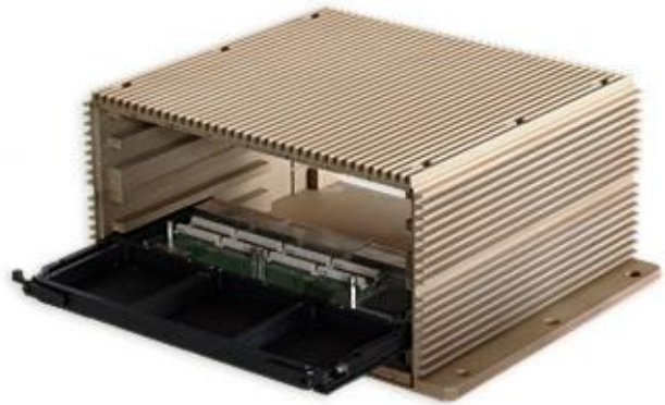
Figure 5: Boards mounted to conduction cards are slid into chassis and locked in place with wedge-locks. The heat must be spread from the rails along the walls to effectively use the natural convection fins that are machined or cast on the external faces.
