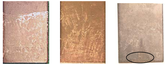
Figure 8 Melonite Coated 304 SST Samples Wetting only on 8-week sample at scribe mark.
