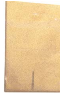
Figure 4 – Typical Test Specimen with Scribed Mark
