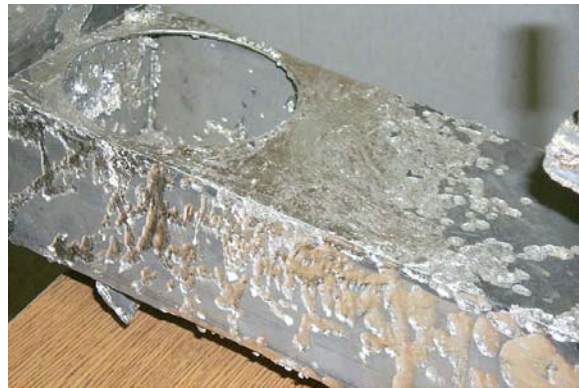
Figure 1 – Failed Stainless Steel Solder Flow Duct
