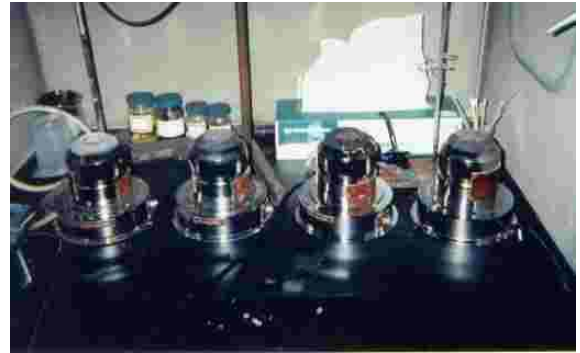
Figure 3 – Solder Exposure Baths
