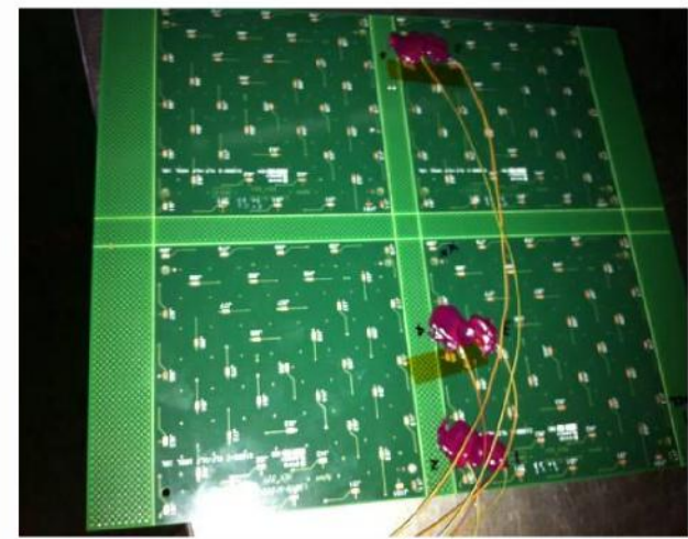
Fig.2: Thermocouples mounted on a profile board
