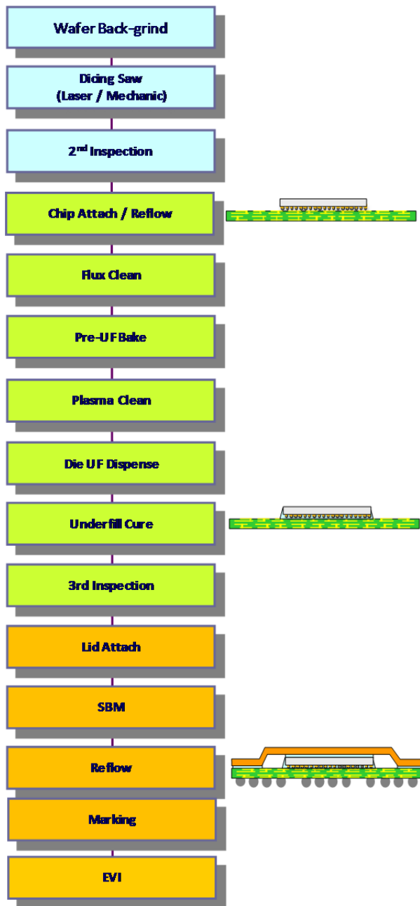
Figure 3: Typical assembly flow for standard flip chip BGA (fcBGA) package
