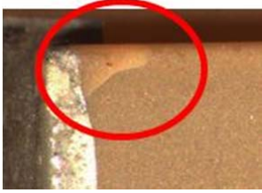
Figure 10. Drop/Shock Test Crack Failure on Surface Mount X7R
