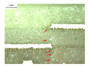
Figure 3. An example of crack propagation through the dielectric of a module experiencing DTC environmental stressing. The red arrows indicate the path of the crack.
