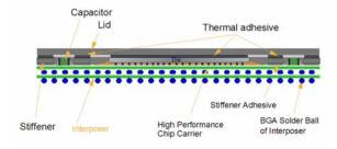
Figure 5. This is a cross-sectional diagram view of the module mounted on the interposer (not to scale).
