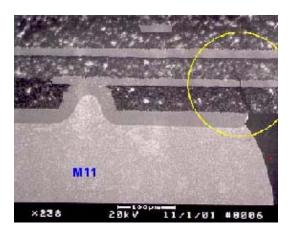
Figure 4. An example of crack propagation through the dielectric of a module and circuit line experiencing DTC environmental stressing resulting in an electrical open and test failure, highlighted in the yellow circle.
