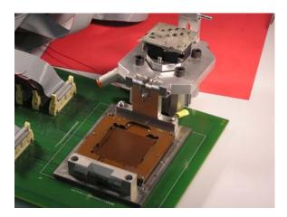
Figure 7. This is a picture of the open clam shell socket test fixture.
