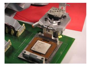
Figure 8. This is a picture of the 52.5 mm FCPBGA-HP module / interposer assembly test vehicle in the open clam shell socket test fixture.
