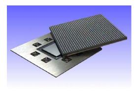
Figure 1. This is an image of a FCPBGA-HP module without lid from top view and bottom view.
