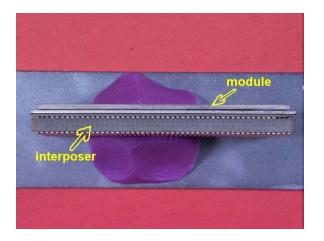
Figure 6. This is a picture of the 52.5mm FCPBGA-HP module / interposer assembly test vehicle.
