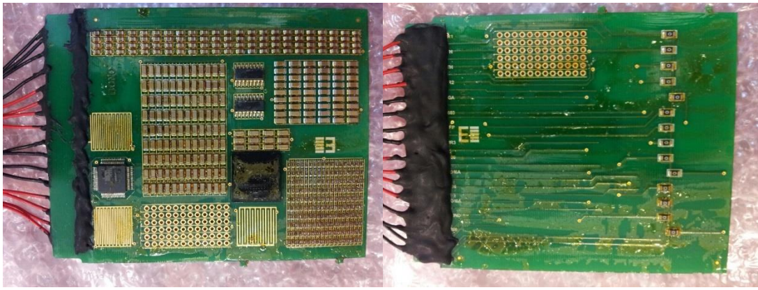
Fig 7. Soldering and Potting of interconnects
