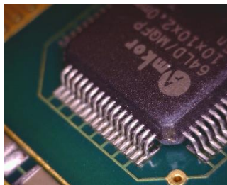
Fig 4. QFP leads at alternating polarity.
