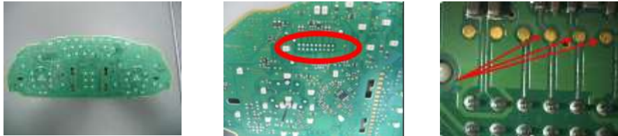
Figure 1: Printed circuit board with flux affected test point around connector area.
