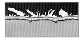
Intermediate growth begins at the plating-underplate/substrate boundary and moves outward.
