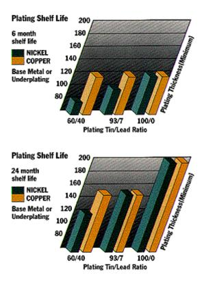
Eventually an intermetallic grows to the surface of the plating, where it oxidizes. An oxidized intermetallic layer will not solder.
