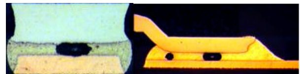
Figure 9: Solder Voiding in Package D Assembly – Left: Front Cross-sectional View, Right: Side Cross-sectional View [5]
