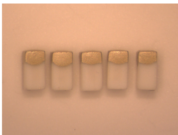
Figure 19. Paste C1 with reduced V1 in the formulation exhibited half-mooning
