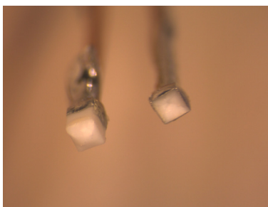
Figure 18. Adhesion failure mode for B4 was ceramic failure.
