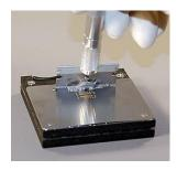
Fig 7. Printing Solder Paste on QFN device while in holding tool
