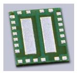
Figure 8 Solder paste printed on QFN before placement on PCB for rework
