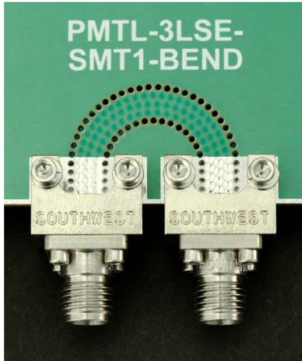
Figure 15: PMTL bend analysis structure.
