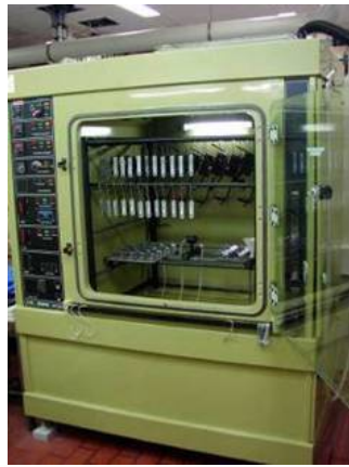
Fig. 7 Salt-Spray Test Chamber
