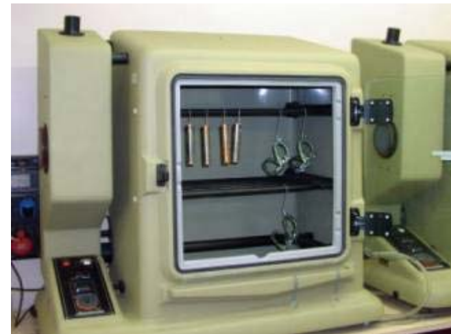
Kesternich – test chamber
