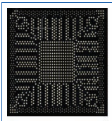
Figure 1. Chipset BGA with an 0.8 mm ball pitch and 0.358 mm ball diameter.
