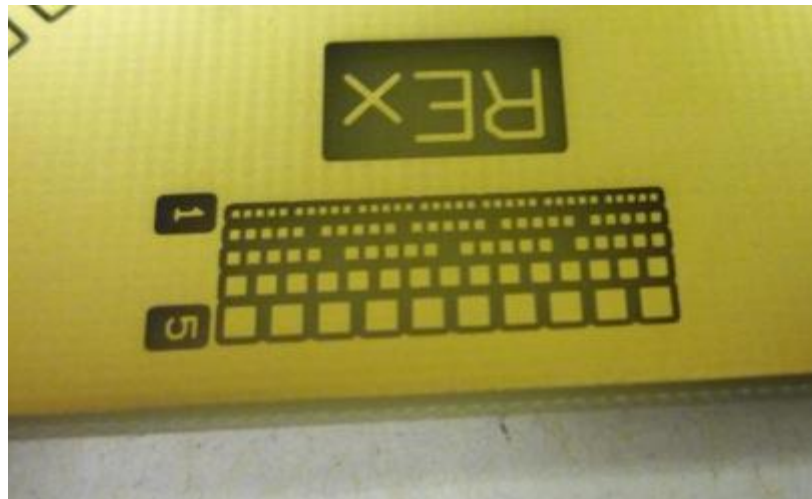
Figure 5 - Test pattern used at the left/right and front/back sides of the reference board.
