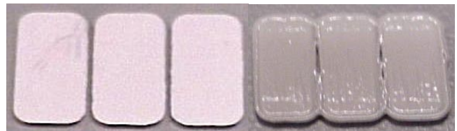
Fig.9 Comparison of Clean Print (Print #1) Resulting in No Voids (Left) and Wavy Top Surface (Print #5) Resulting in Numerous Voids (Right)
