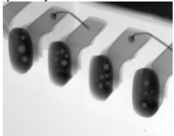
Image 16: Acceptable Condition of QFN edge joints showing an increased level of voiding within the joints but well within any action level.
