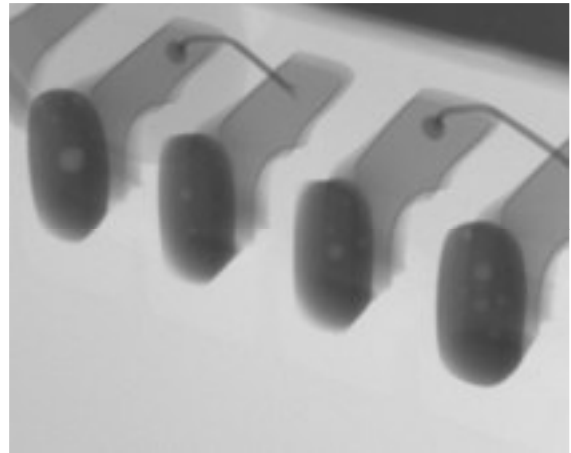
Image 15: Target Condition of QFN edge joints where showing a moderate level of voiding within joints is acceptable. All joints have reflowed.
