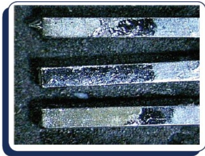
Figure 7-2 Dip & Look solderability testing of transformer leads without ROSA treatment (top) and after ROSA treatment (bottom)
