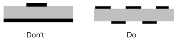
Figure 2. Example of copper spreading on flex
