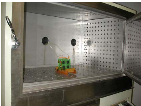
Figure 7- Test boards in Thermal Cycle Chamber
