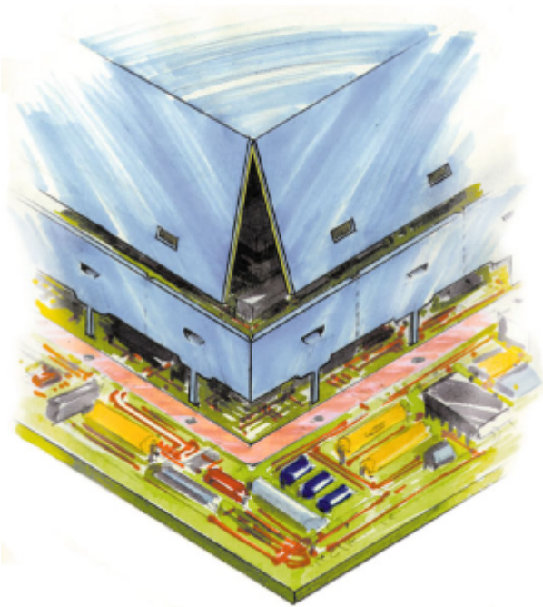
Figure 19.2: Fixed part on the PCB (2. fence) and a separate cover (1)
