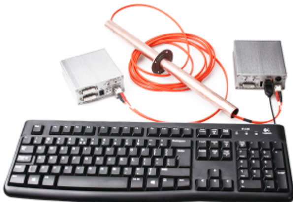
Figure 65.1: Example of a fiber optic converter combined with a waveguide
