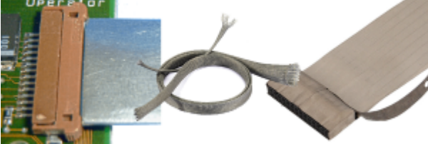
Figure 21.1: Flat cables, round cables, bundles of cables and branches can be shielded
