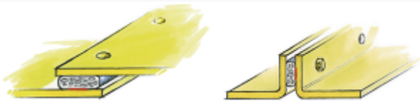
Figure 42.1: Examples of gasket solutions for small constructions
