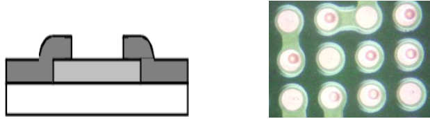
Figure 1 – Solder Mask Defined Pad
