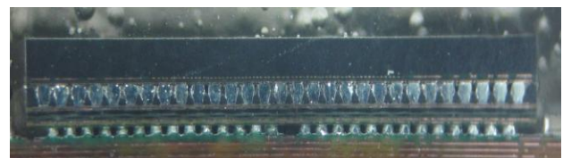
(b) X-section of POP using SMT 256
