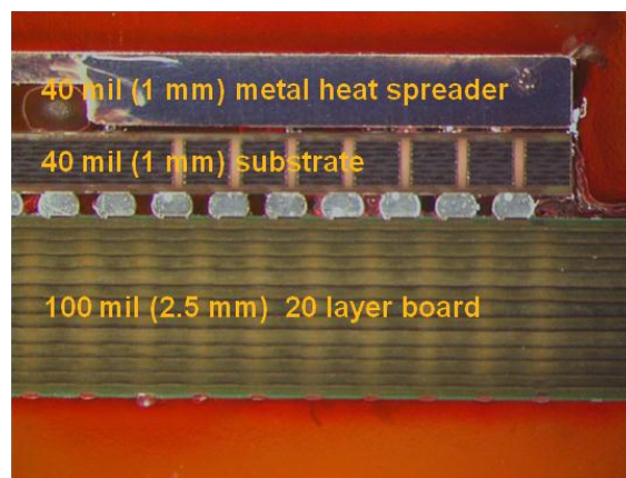
Figure 4: Typical structure- 40 mm pkg on 20 layer board
