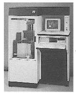
Using a computer, ultraviolet laser, and vat of UV-curable polymer, stereolithographic models are produced in a fraction of the time and cost.
